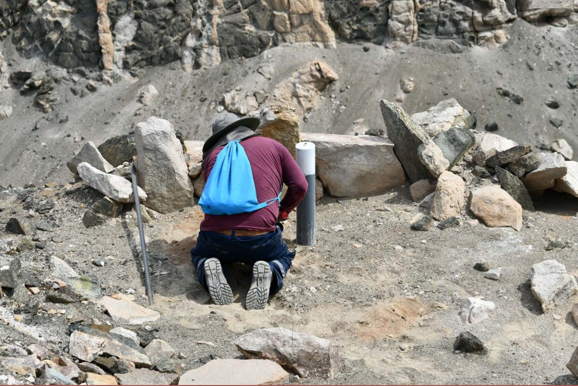
Figures: Total station and GPS RTK measurements (establishing and stabilizing control points).
